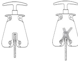
The unit itself must never be used as a means for attaching ropes, chains or belts.
