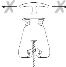
Always insert the load fully into the mouth of the clamp.
