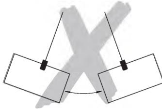
Only one sheet metal plate may be transported at a time with the load lifting attachment.
