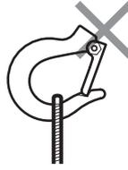
Improper hooking position of the lifted load or the sling
