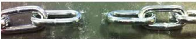
2. Make sure the chain is not twisted and bring the two ends together.
