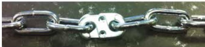
4. Fix the two halves of the speed link together with two 2.4mm x 6mm stainless steel pop rivets.
