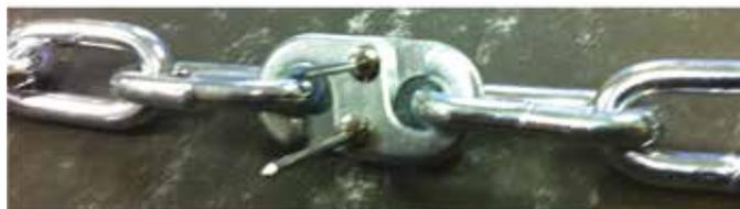
**Note:** The indicated 'speed links' must only be used on hand chain which fully complies with the dimensional detail indicated within this script. The hand chain runs over a specific calibrated pocket wheel and the chain is also calibrated to suit this particular pocket wheel.
