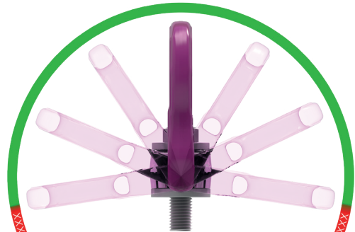
Pic. 10: Pivoting area (green = permitted loading direction)
