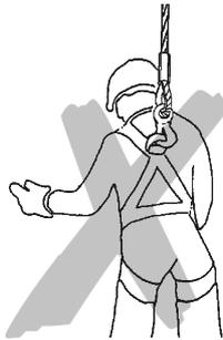
Performing welding jobs on the lifting unit, the rope drum and the rope is prohibited. The rope should never be used as an earth connection during welding.
