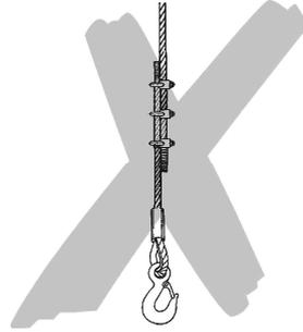
The loose end of the rope must not be used for attaching loads.
