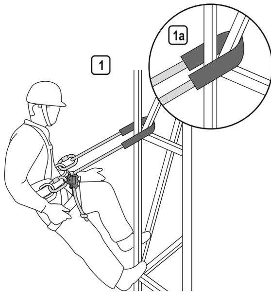
2. The device can be attached to attachment buckle of a sit harness compliant with EN 813 or a single D-ring of a work positioning belt – Fig. 2. Attach connector for rope length adjuster to attachment buckle of a harness, and rope connector to anchor point located at the height of user's waist or above. Shape and construction of anchor point must not allow for a self-acting disconnection of the device. Minimal static strength of anchor point should be 12kN.
