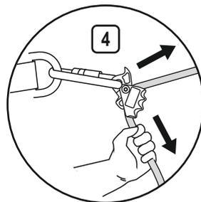
NOTE: Before and during operation, check whether individual attachment elements are connected properly. Connectors must be closed and protected against accidental opening by locking gear.
