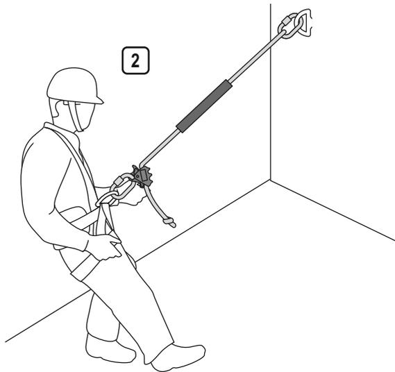
3. Using the rope adjuster, adjust the length and the tension of the rope to assure a stable work position and restrict the free fall of the worker. The lanyard must be kept taut during use.
