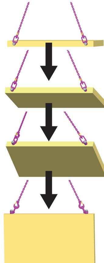
Pic. 5: Possible turning operation with the VLBG-PLUS
